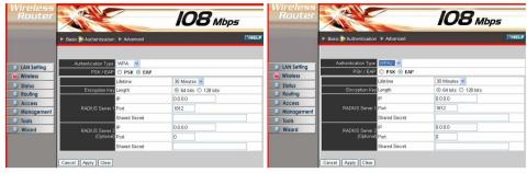
If WPA or WPA2 is selected, the below screen is shown. Please set the length of the encryption key and the parameters for the RADIUS server.
